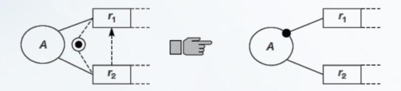
The two constraints in the first model says: each A must play r1 or r2 (or both), and that if A plays r2 then it must play r1. This means that r1 must be always played (which is the second model)
