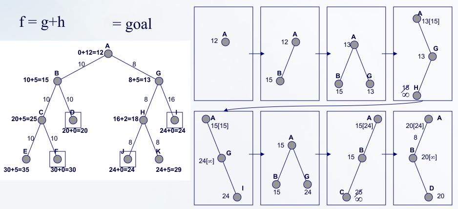
$\infty$  is given to nodes that the path up to it uses all available memory. Can tell when best solution found within memory constraint is optimal or not.
